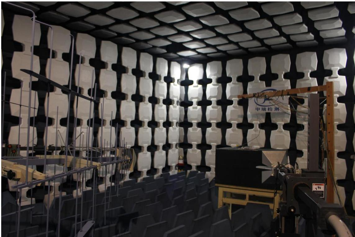
The radiated emission tests were performed in the 3-meter Chamber, using the setup accordance with the FCC part 2.1053. The specification used was the FCC 2.1053 limits.
