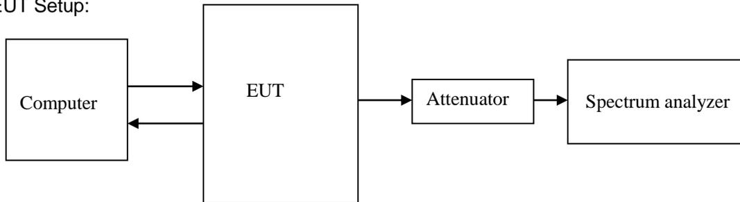
REMARKS: Attenuator loss (dB)=30dB, Cable Loss (dB)=1.5dB.
