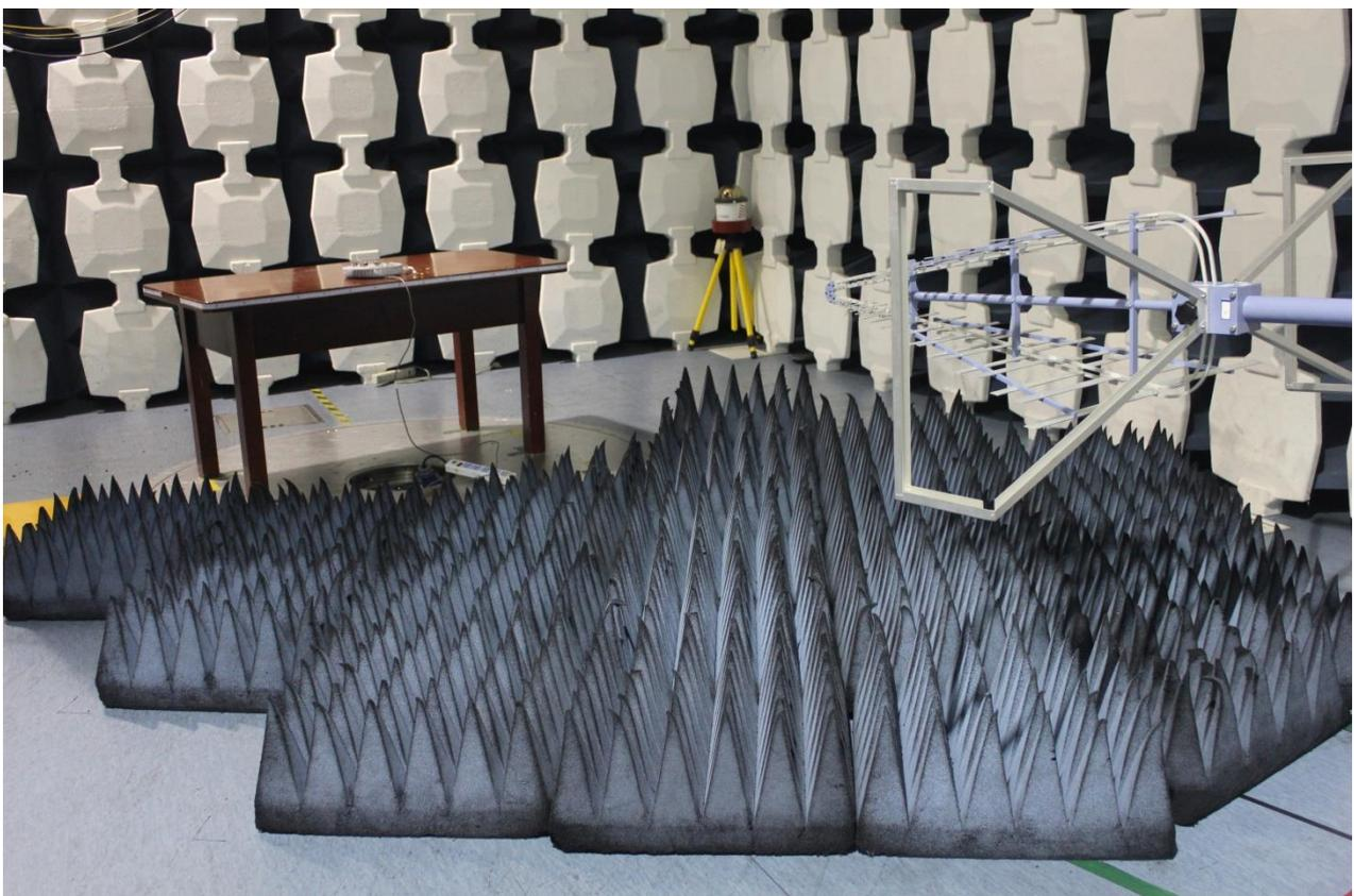
Fig.2 Radiated emission test (above 1 GHz)
