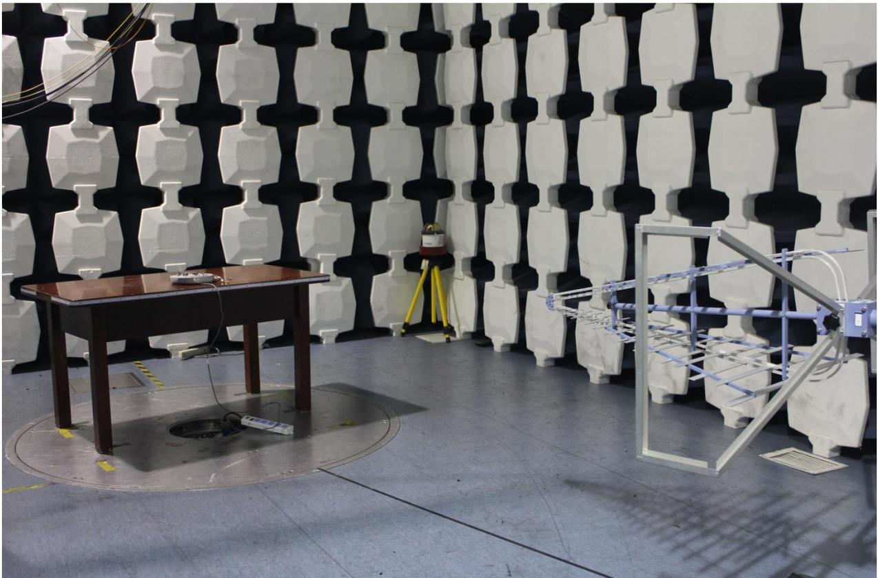
Fig.1 Radiated emission test (below 1 GHz)
