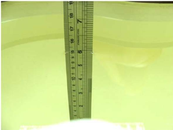
Fig 6.1 Photo of Liquid Height for Head SAR
