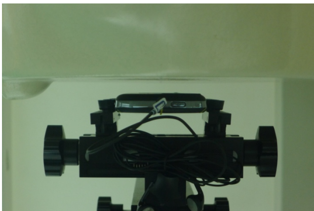
Back of the DUT with Phantom 1 cm Gap (w/headset)
