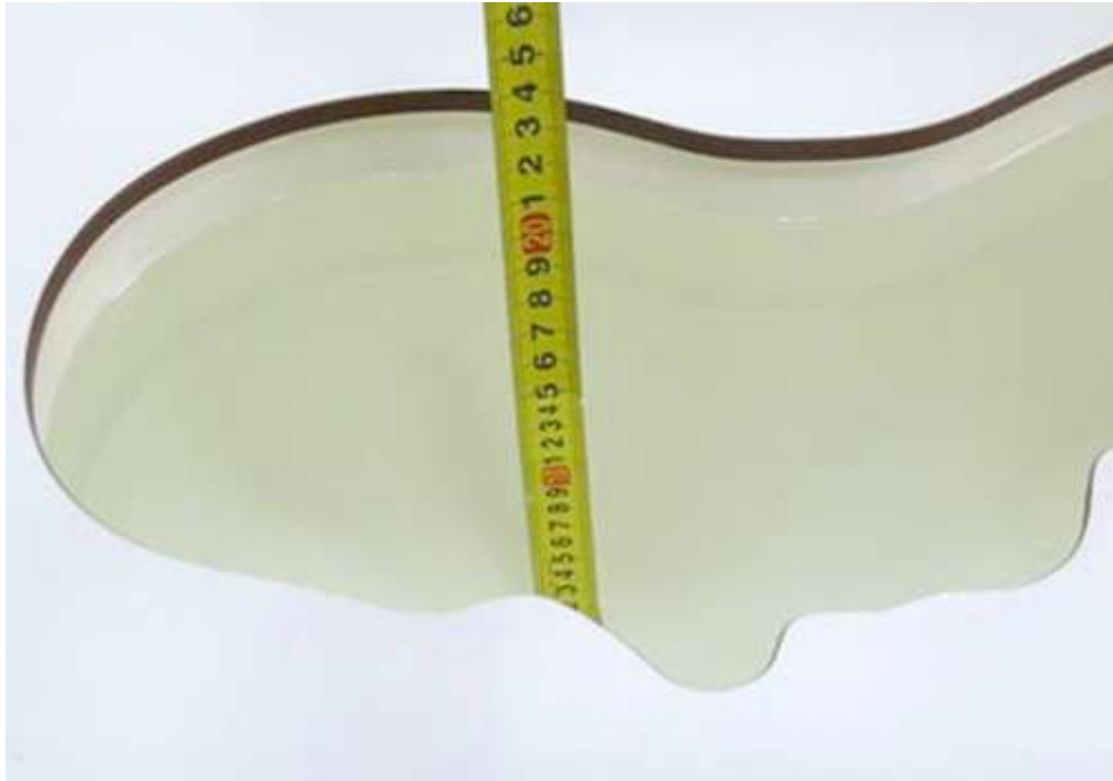
Picture 5: liquid depth in the head Phantom (1900 MHz) (15.2cm deep)
