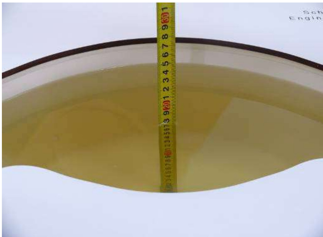
Picture 2: Liquid depth in the flat Phantom (900MHz) (17.5cm deep)
