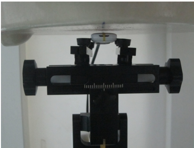
USB Cable Plug-in for USB Configuration 2 (Horizontal Down with Phantom 5 mm Gap)
