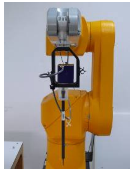
Figure 3. ES3DV3 E-field probe
