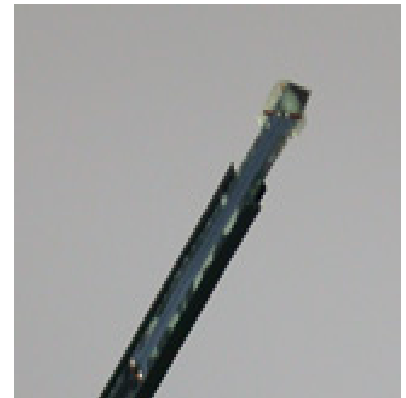
Figure 2. ES3DV3 E-field Probe
