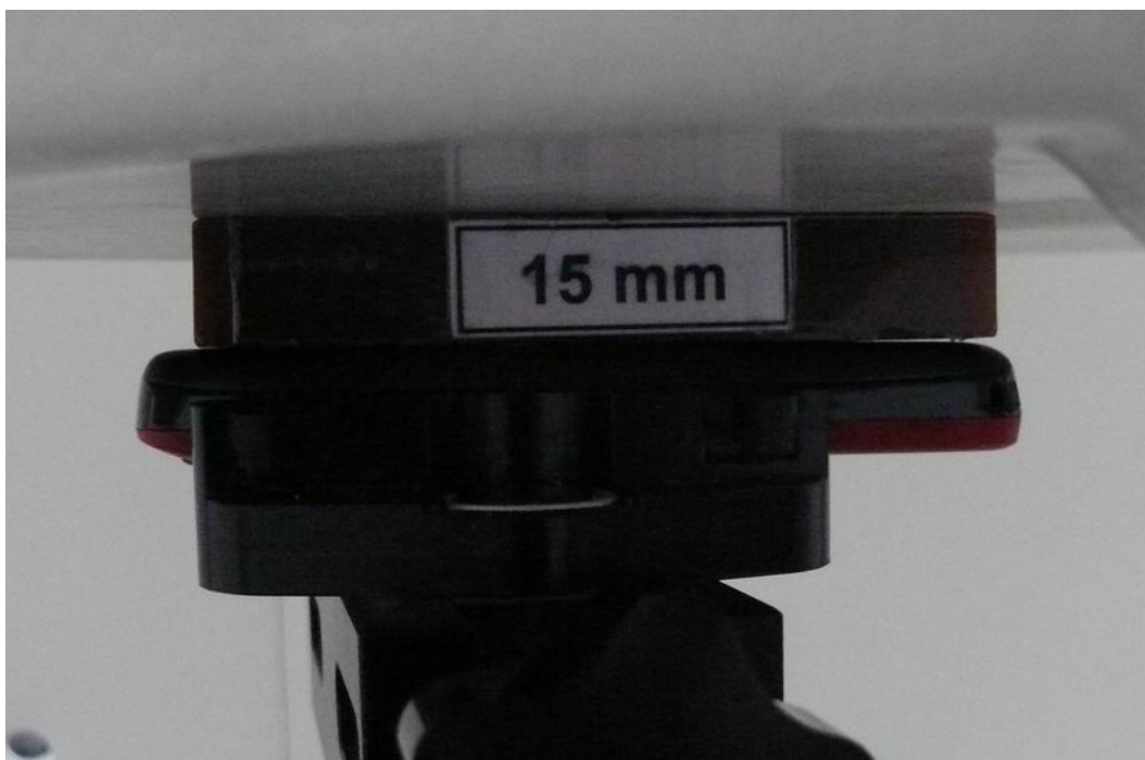
Picture 11: Body, The EUT display towards ground, the distance from handset to the bottom of the Phantom is 15mm (The spacer was removed during testing)
