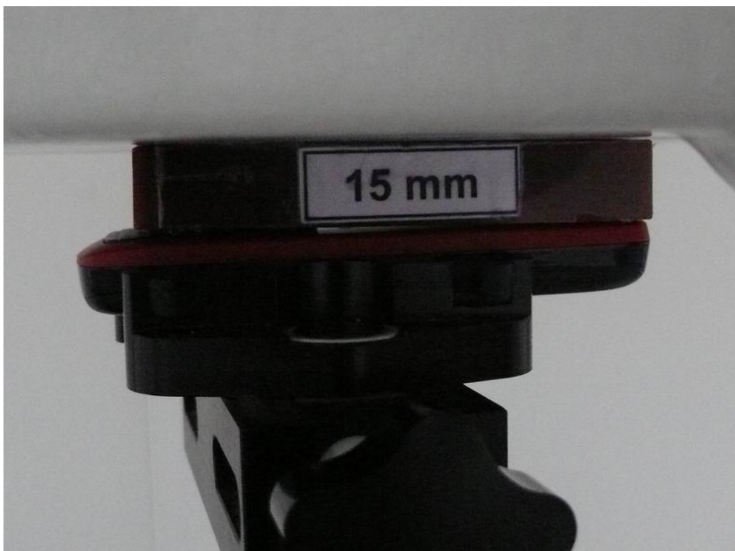
Picture 12: Body, The EUT display towards phantom, the distance from handset to the bottom of the Phantom is 15mm (The spacer was removed during testing)
