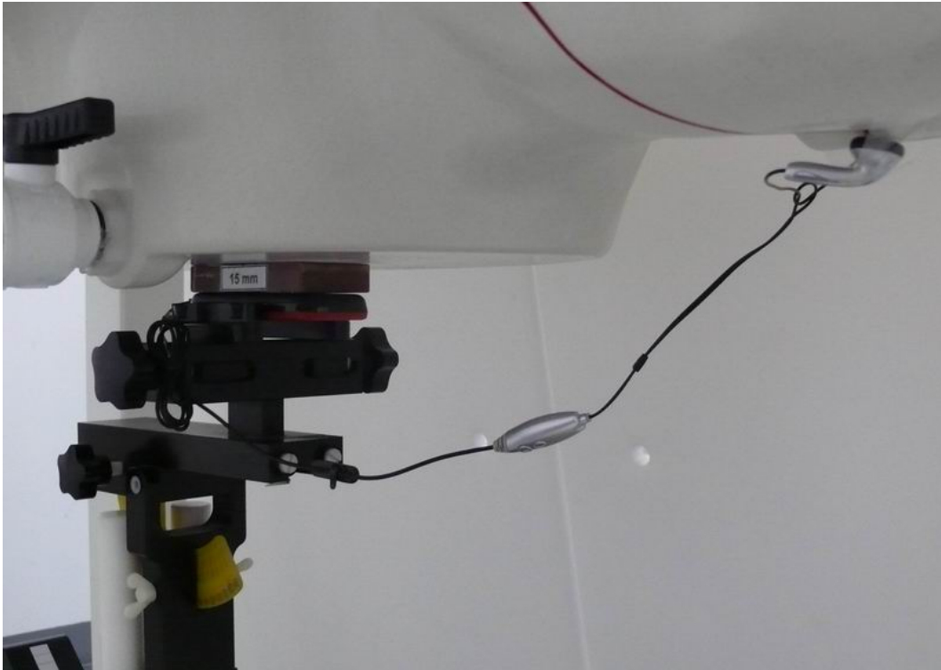
Picture 13: Body with earphone, The EUT display towards ground, the distance from handset to the bottom of the Phantom is 15mm (The spacer was removed during testing)
