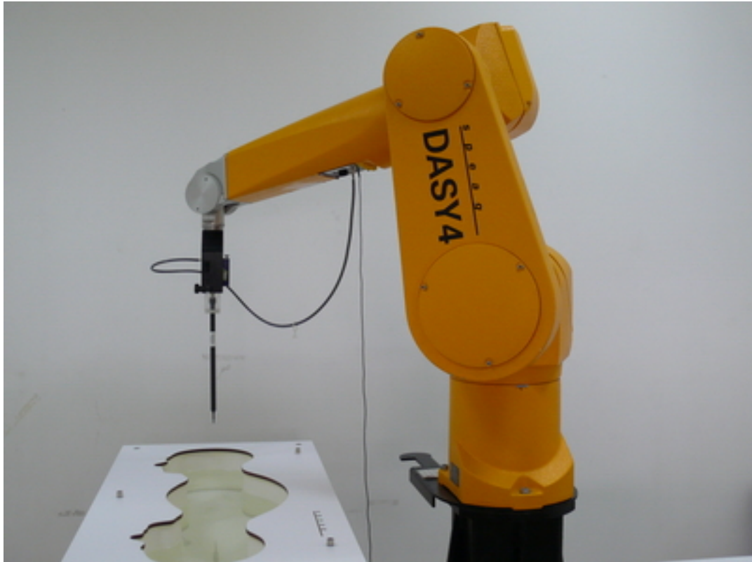
Picture 1: Specific Absorption Rate Test Layout
