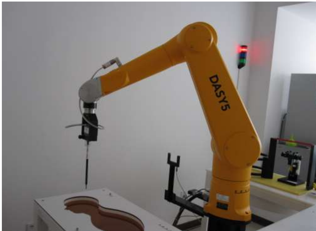
Picture 1: Specific Absorption Rate Test Layout
