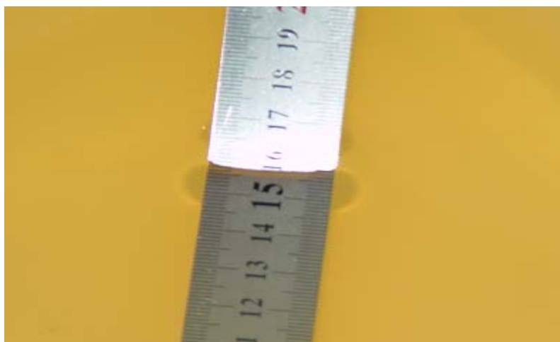
Liquid depth for SAR Measurement
