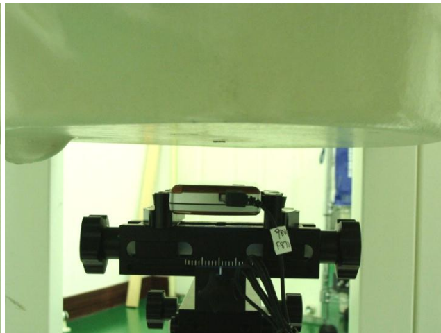
Bottom of the DUT with Phantom 2.5 cm Gap for Slide Off Mode
