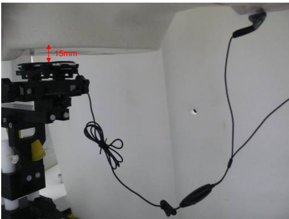
Picture 16: Body with earphone, The EUT display towards phantom, the distance from handset to the bottom of the Phantom is 15mm
