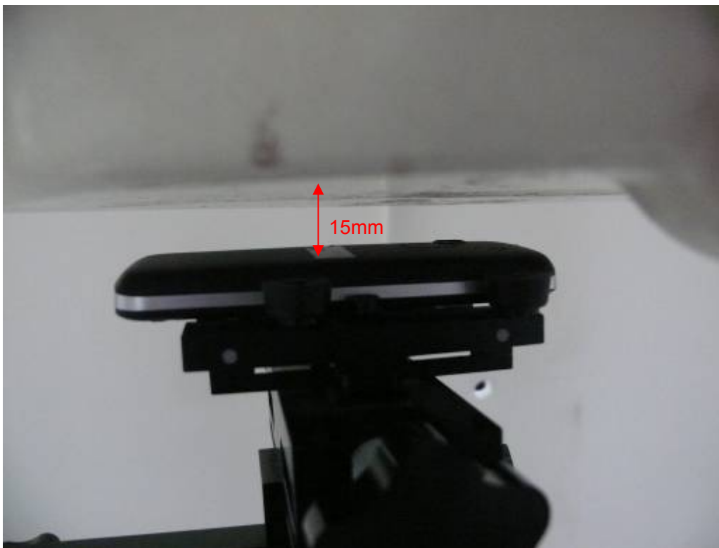
Picture 13: Body, The EUT display towards ground, the distance from handset to the bottom of the Phantom is 15mm
