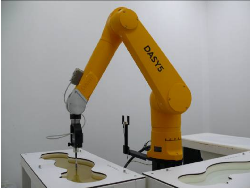
Picture 1: Specific Absorption Rate Test Layout
