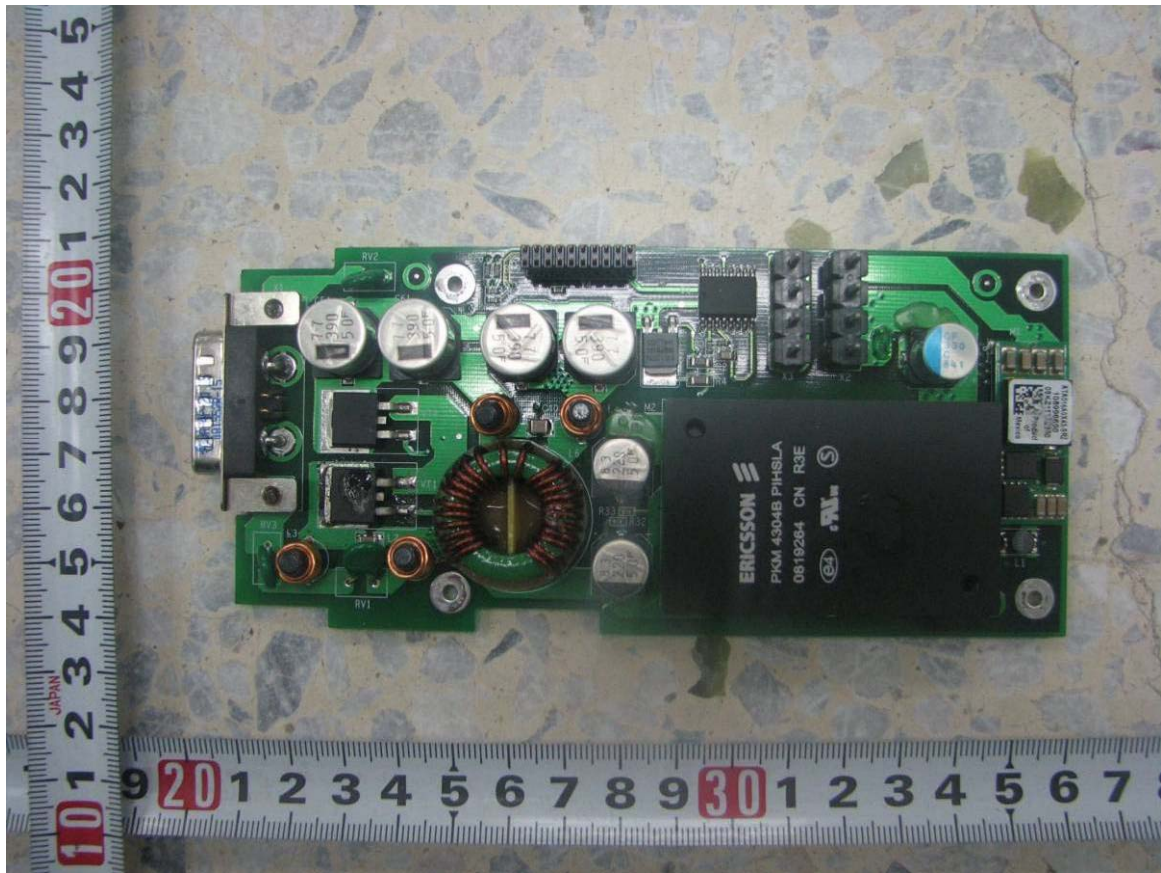
view of the power supply module
