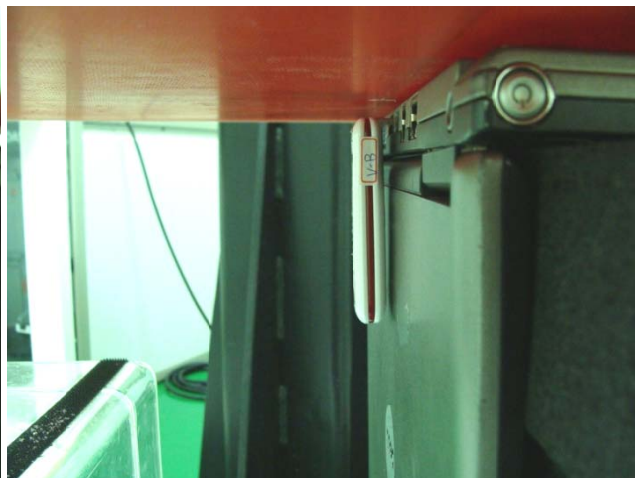
USB Configuration 1 (Horizontal Up) Vertical mode with Phantom 5 mm Gap
