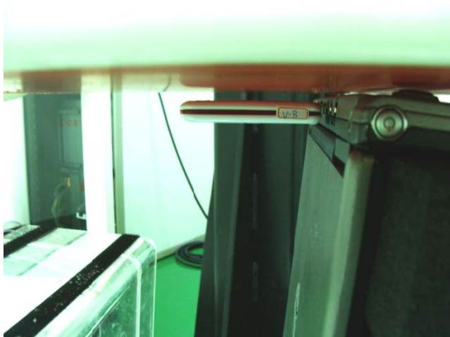
USB Configuration 1 (Horizontal Up) Straight mode with Phantom 5 mm Gap
