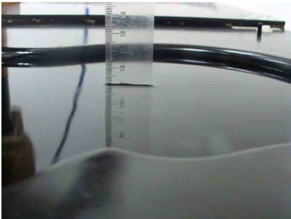
Figure B.2 Depth of Simulating Liquid in SAM Head Phantom
