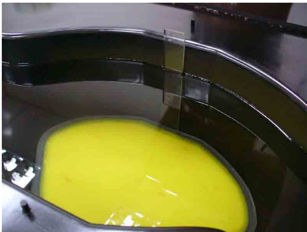
Figure B.3 Depth of Simulating Liquid in SAM Flat (Body) Phantom
