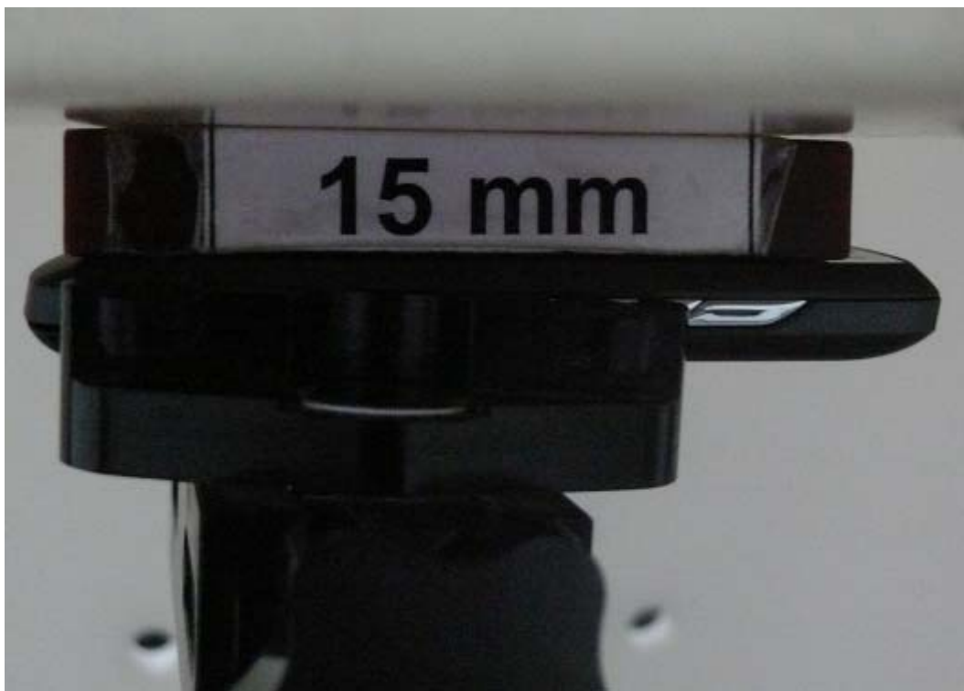
Picture 12: Body, The EUT display towards phantom, the distance from handset to the bottom of the Phantom is 15mm(The spacer was removed during testing)
