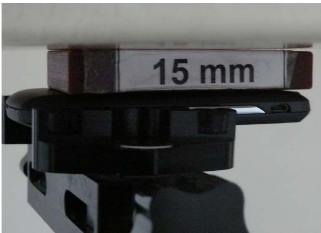
Picture 11: Body, The EUT display towards ground, the distance from handset to the bottom of the Phantom is 15mm(The spacer was removed during testing)
