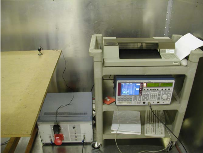
Transmitter Conducted Emission - Front View
