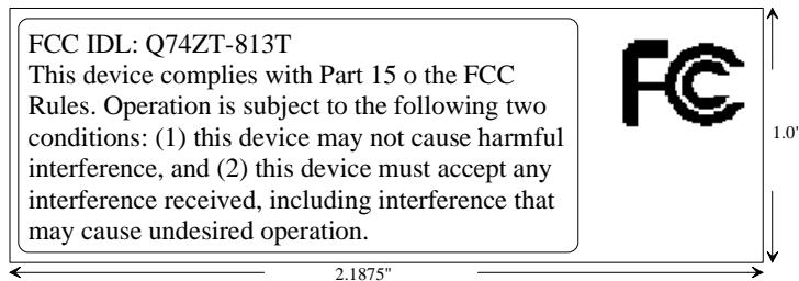
**Specifications:** Text is black or white in color and is left justified. Labels are silk-screened and shall be "permanently affixed" at a conspicuous location on the EUT.
