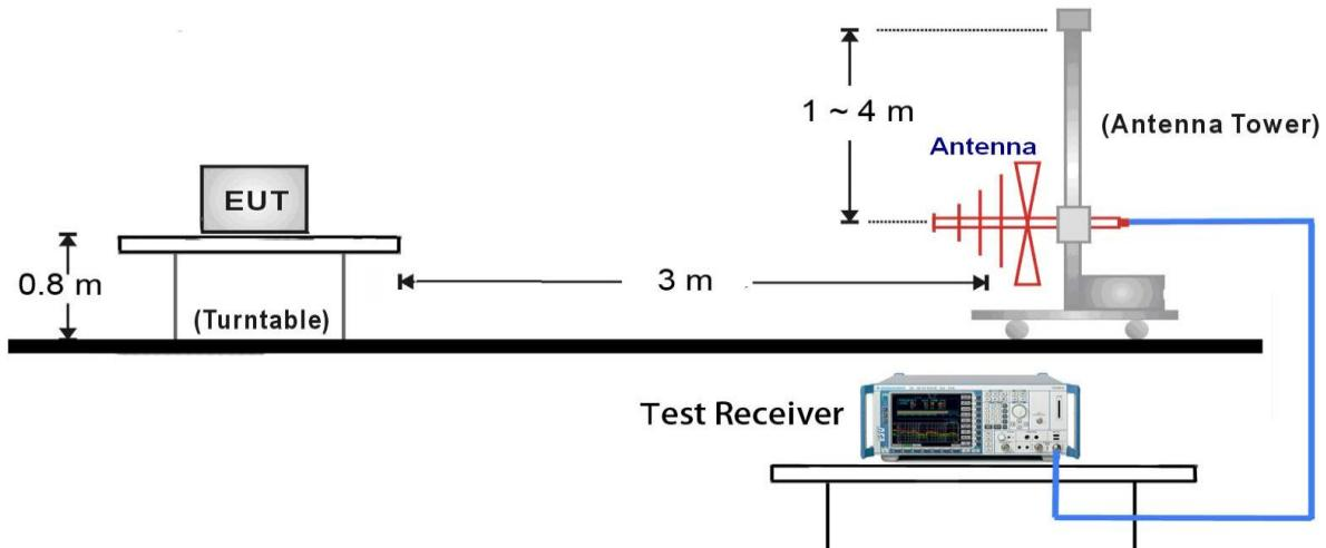
1GHz ~ 40GHz Test Setup:
