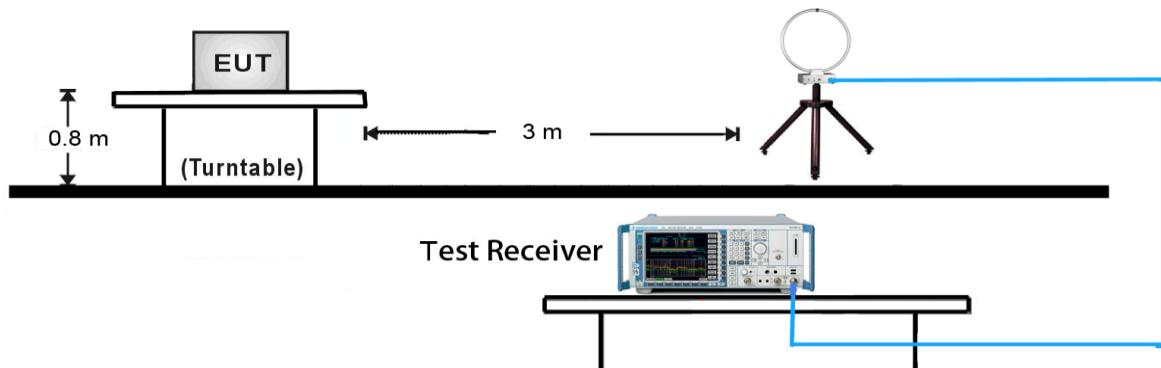
30MHz ~ 1GHz Test Setup:
