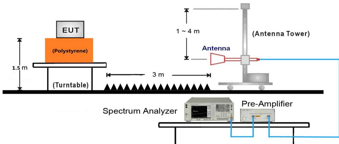
Above 40GHz Test Setup:
