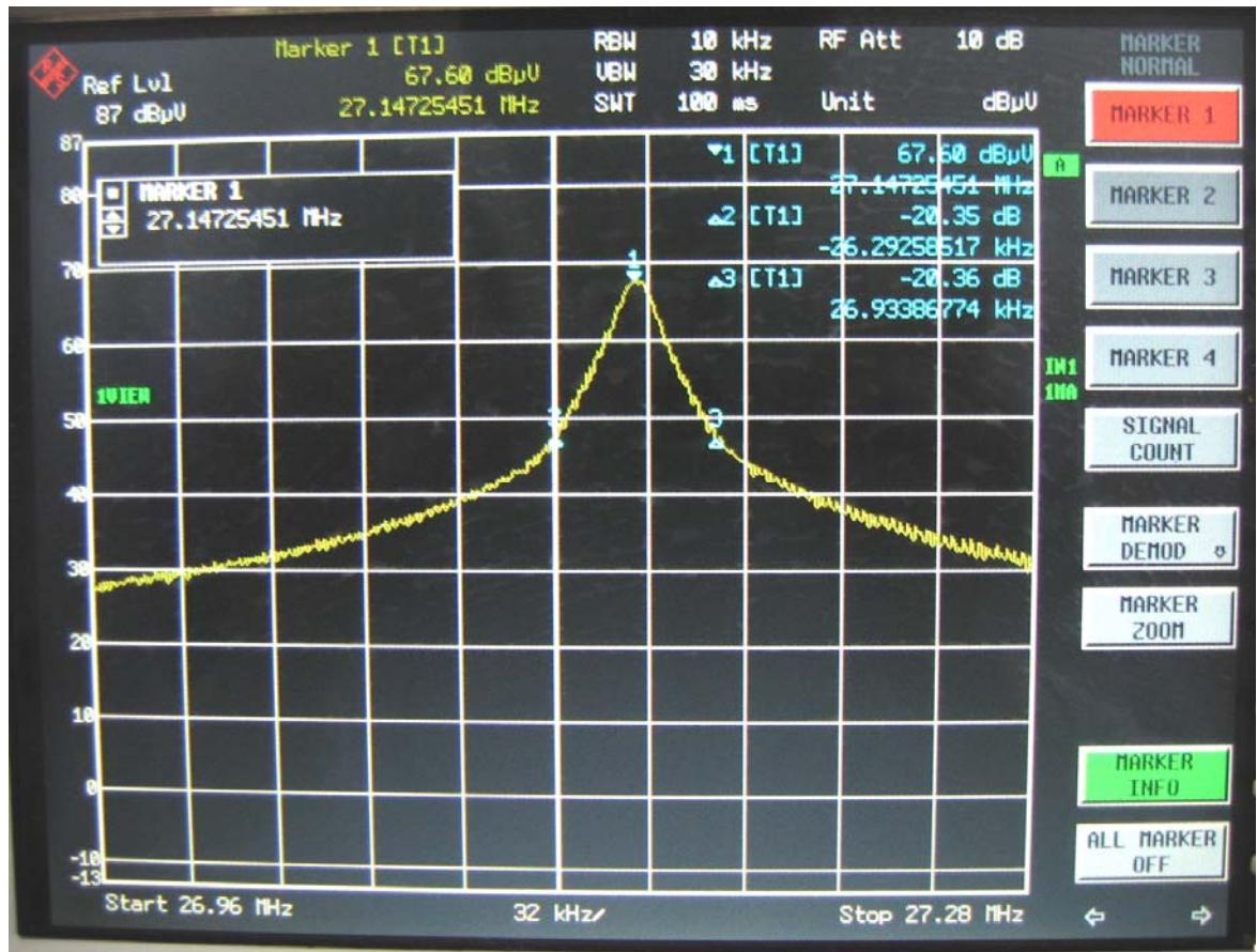
The results: The unit does meet the FCC Part 15 C Section 15.227 requirements.
