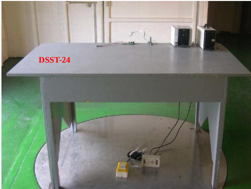
Photo 1: Radiated Emission Test Set-up
