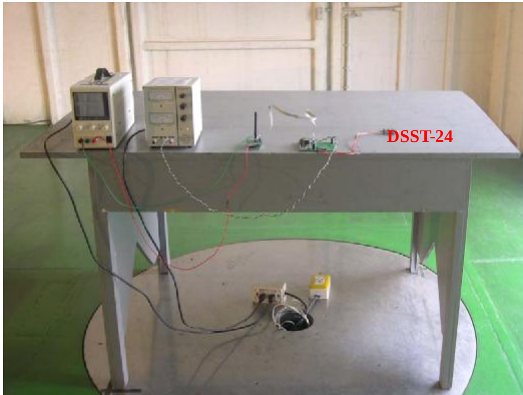
Photo 2: Radiated Emission Test Set-up
