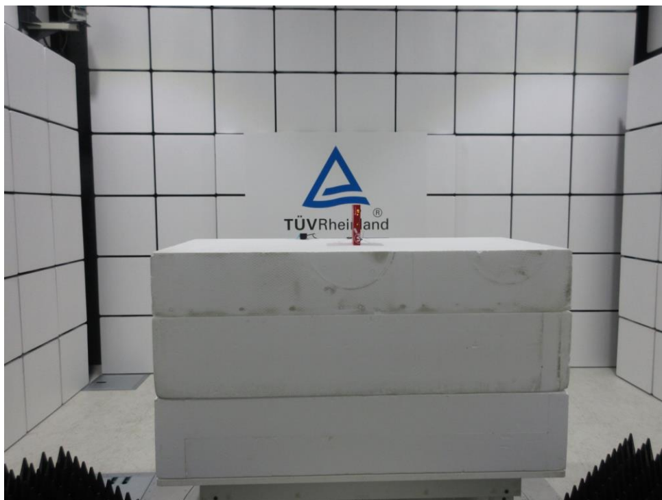
Photograph 2: Set-up for Spurious Emissions (Front View 2)
