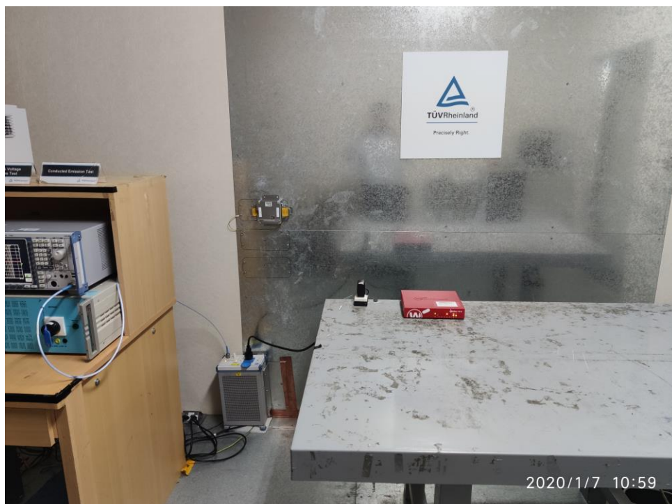
Photograph 6: Set-up for Mains Conducted testing (Front View)
