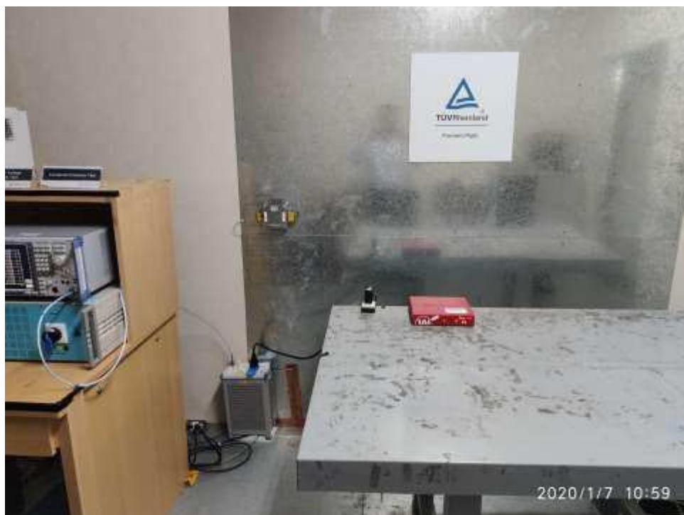
Photograph 6: Set-up for Mains Conducted testing (Front View)
