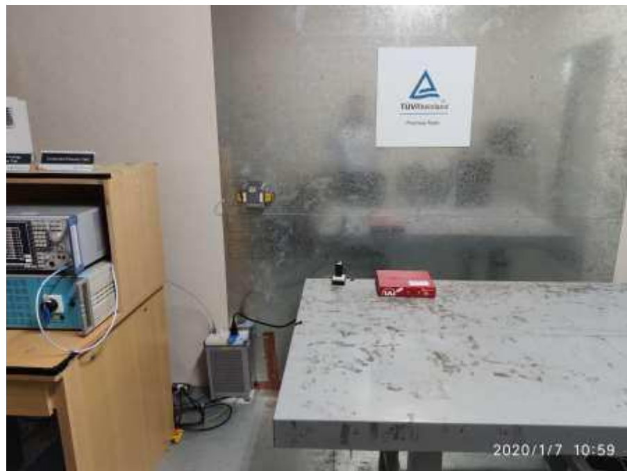
Photograph 6: Set-up for Mains Conducted testing (Front View)
