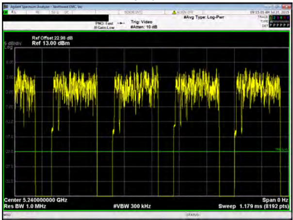
Chain A, 802.11(ac) MCS8 (256-QAM), 20 MHz, High Channel 5240 MHz
