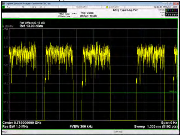
Chain A, 802.11(n) MCS7, 20 MHz, Mid Channel 5785 MHz
