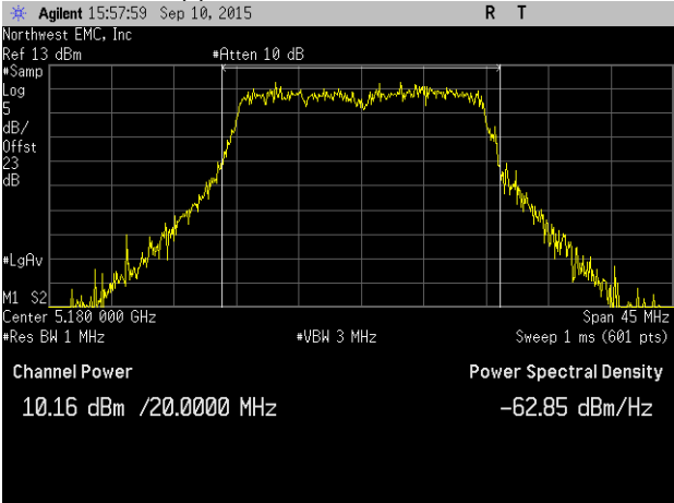
Chain A, 802.11(n) HT, MCS23, 20 MHz, Low Channel 5180 MHz
