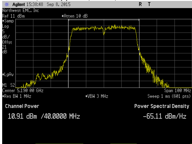
Chain A, 802.11(n) MCS7, 40 MHz, Low Channel 5190 MHz
