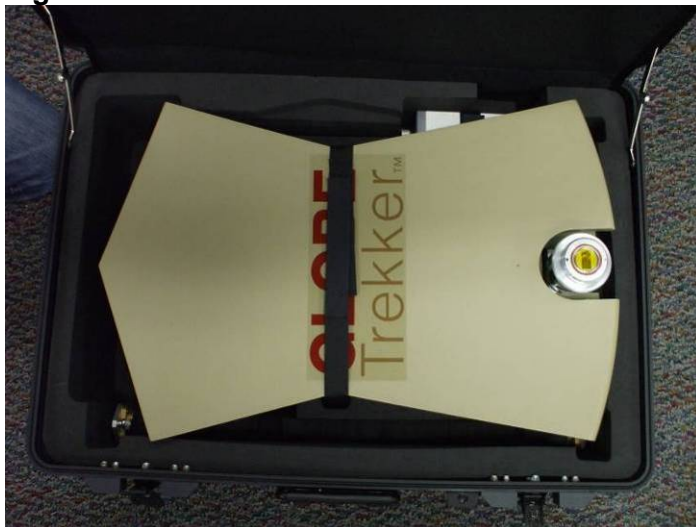
Figure 6. Transit Case A – Main Antenna Unit with Backplate-Mounted SSPA
