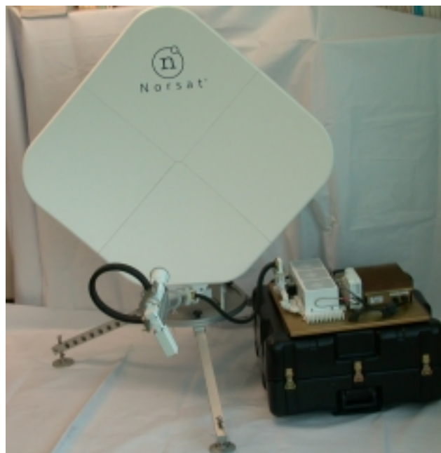
FIGURE 25 Position of SSPA Baseplate and Antenna
