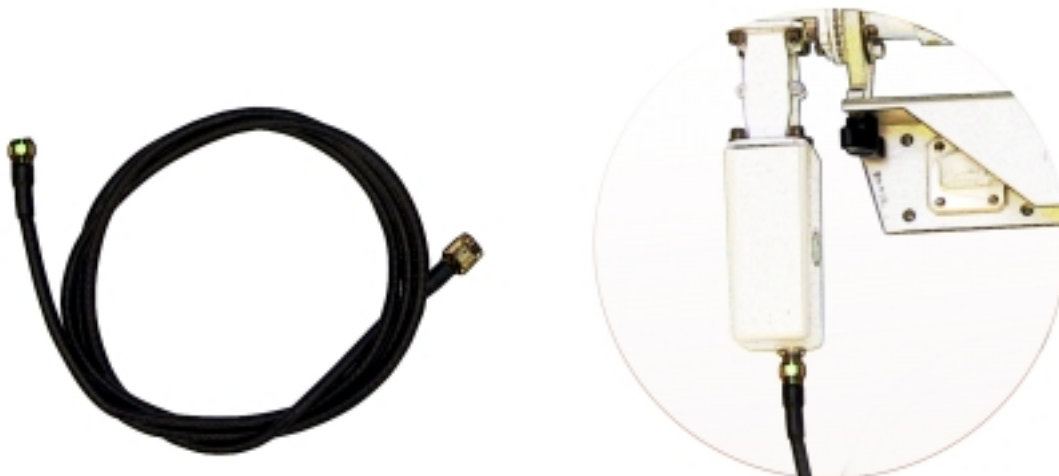
Left: LNB Cable; Right: LNB Cable Connection on LNB
