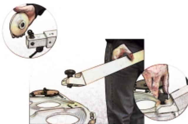
FIGURE 9 Securing Tripod Legs to Support Base
