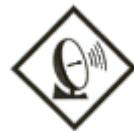
When in operation, i.e., power on, the area directly in front of the antenna reflector must be considered an Area of Restricted Occupancy.
