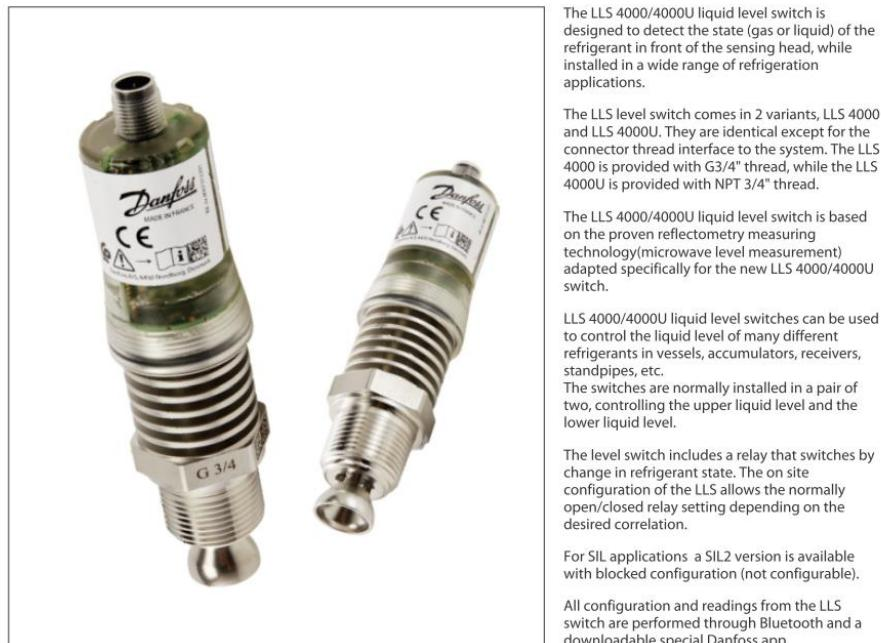
The LLS 4000/4000U liquid level switch is designed to detect the state (gas or liquid) of the refrigerant in front of the sensing head, while installed in a wide range of refrigeration applications.
