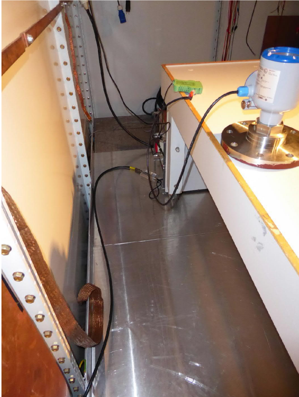
Test AC power line conducted emissions
