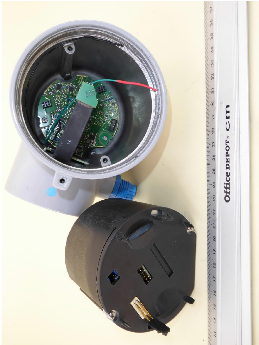
Internal view, converter unit removed
