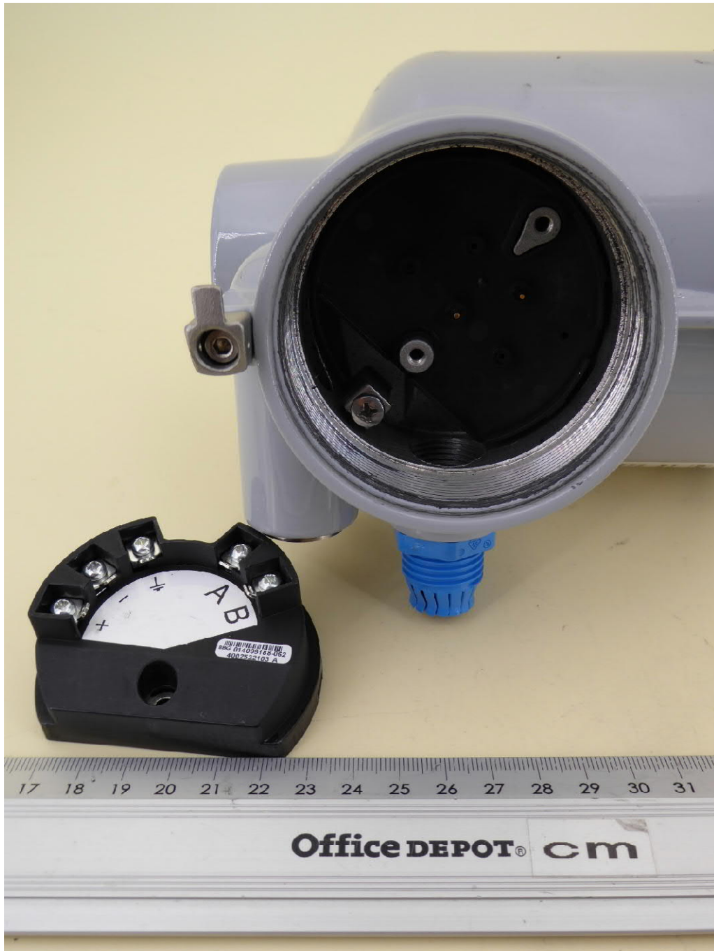
Internal view, terminal board removed
