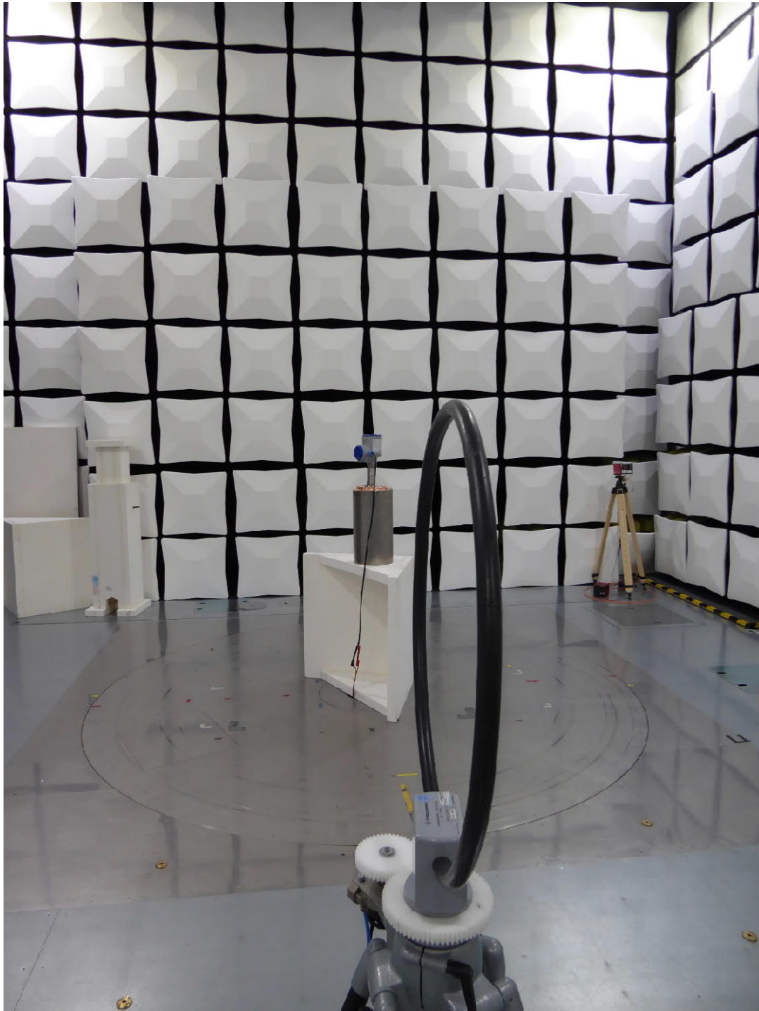
Test setup semi anechoic chamber (<30 MHz)
