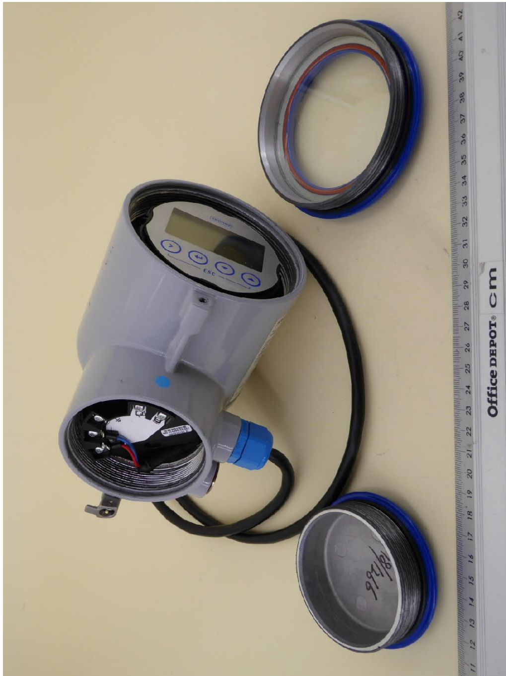
Internal view, housing opened
