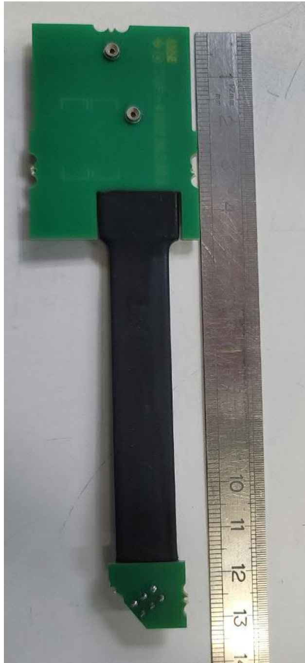
Connector PCB, top view (photo supplied by the applicant)
