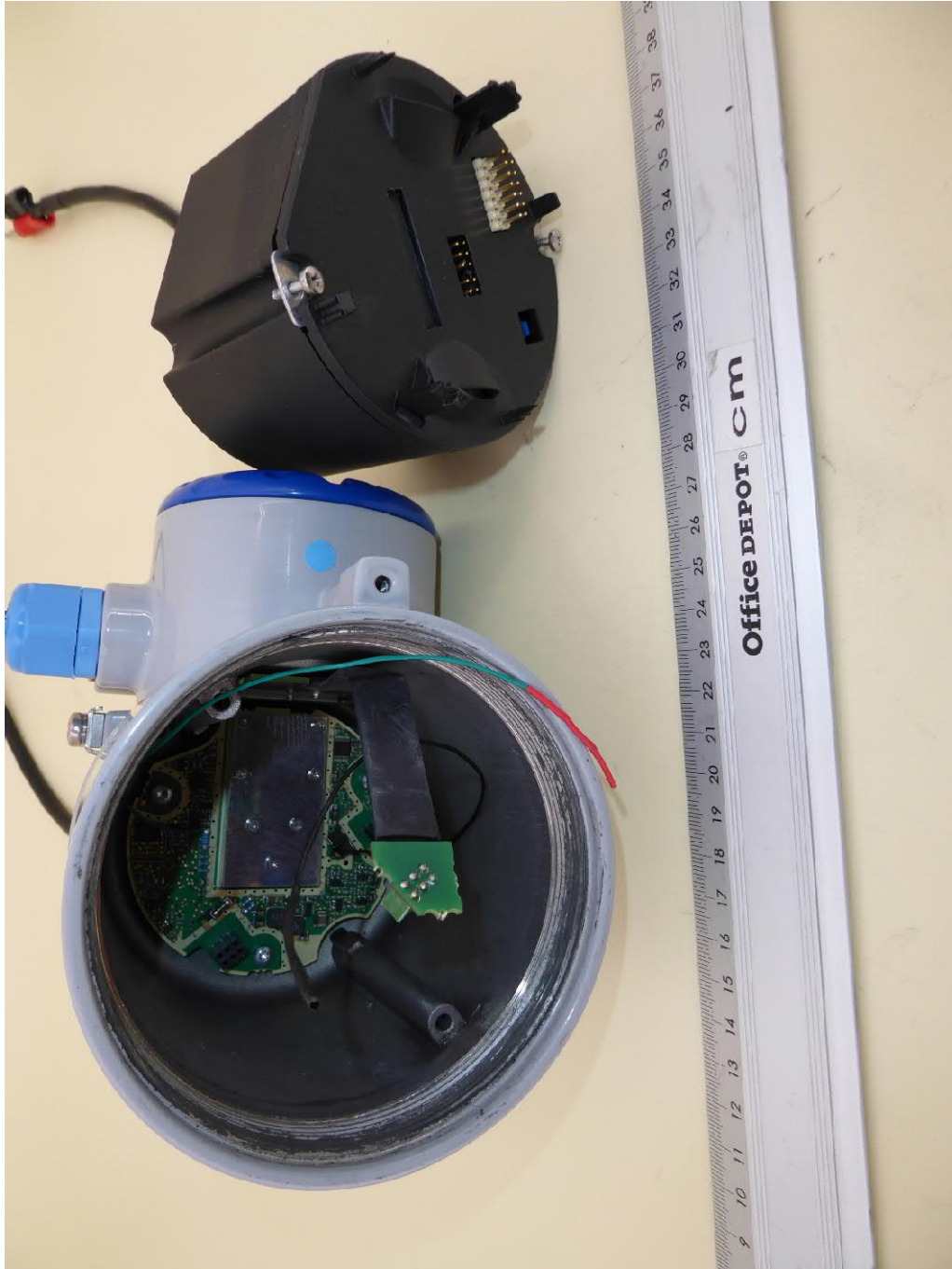
Internal view, converter unit removed
