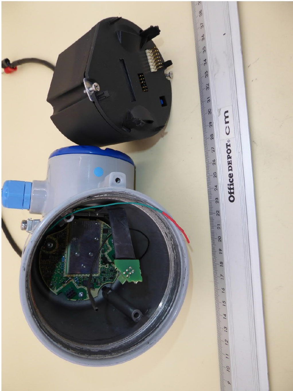
Internal view, converter unit removed
