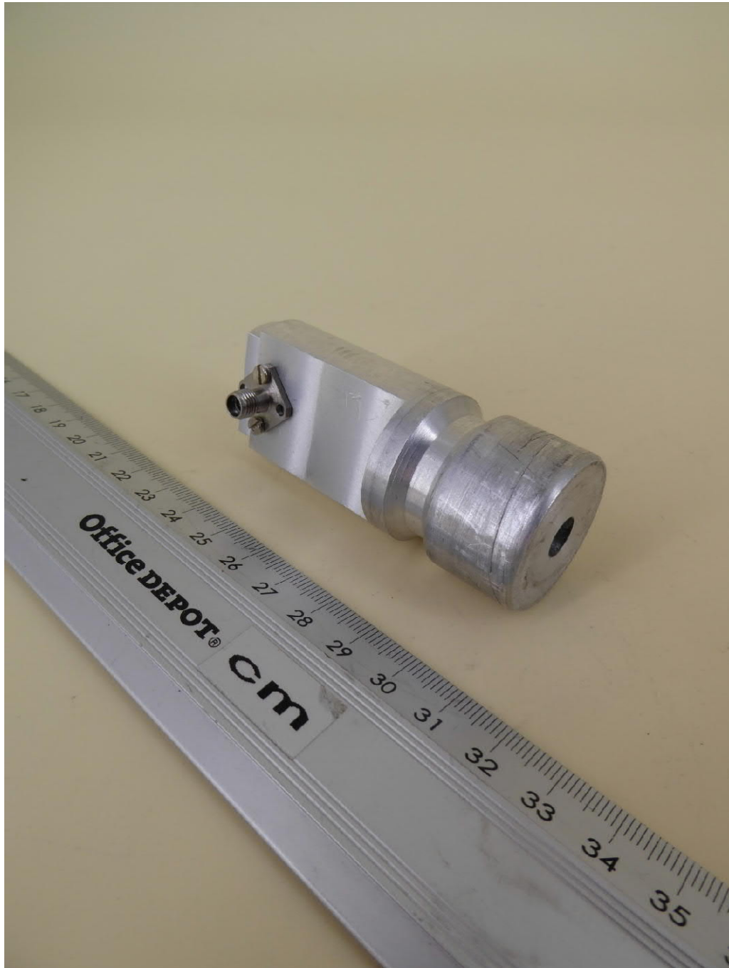
RF-adaptor used for conducted measurements, 3-D-view
