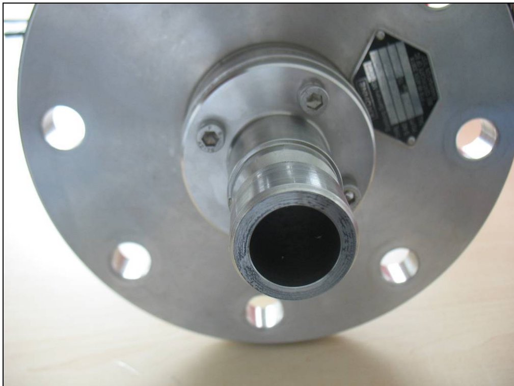
Photo 14: Metallic Horn Antenna
