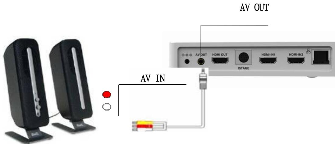
Notes: Do not connect the yellow wire when AV wire is connected to Media Sounder.
