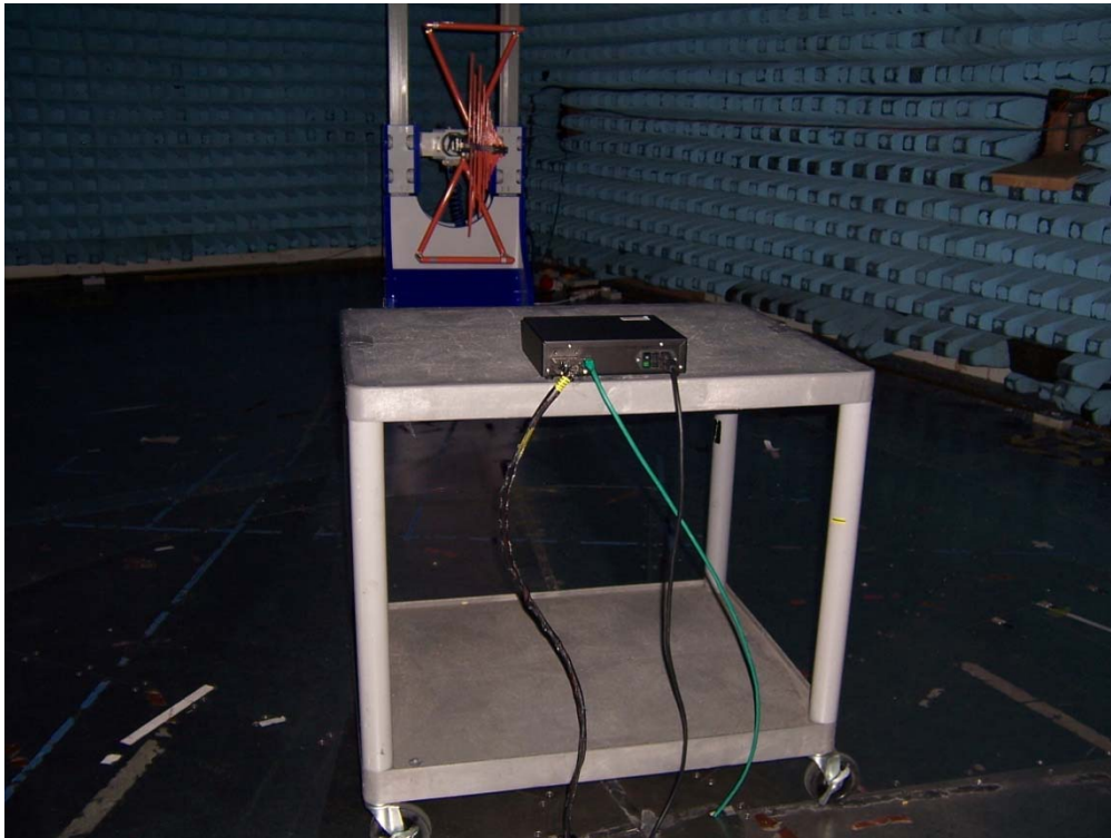
Figure 7 - Test Setup – Radiated Emissions Below 1 GHz
