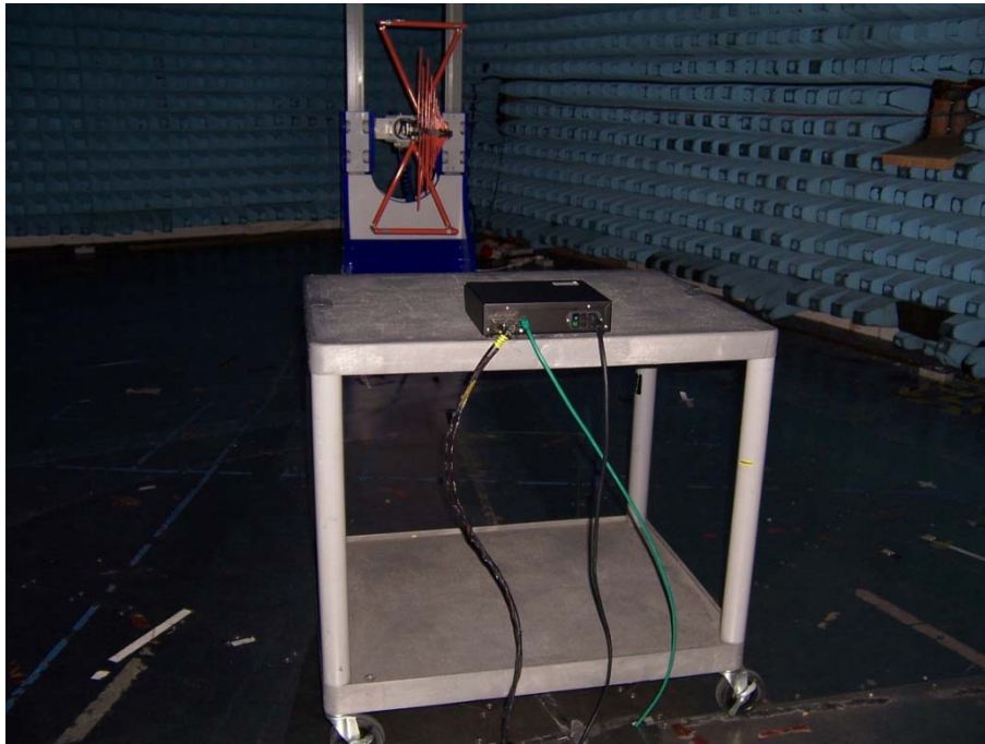
Figure 4 - Test Setup – Conducted Emissions
