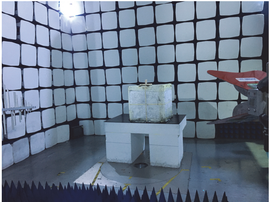
Radiation Emission Test Setup (1GHz to 18GHz)
