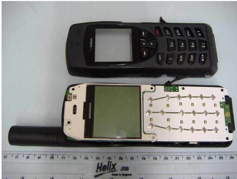
Front Overview Case Front Removed
