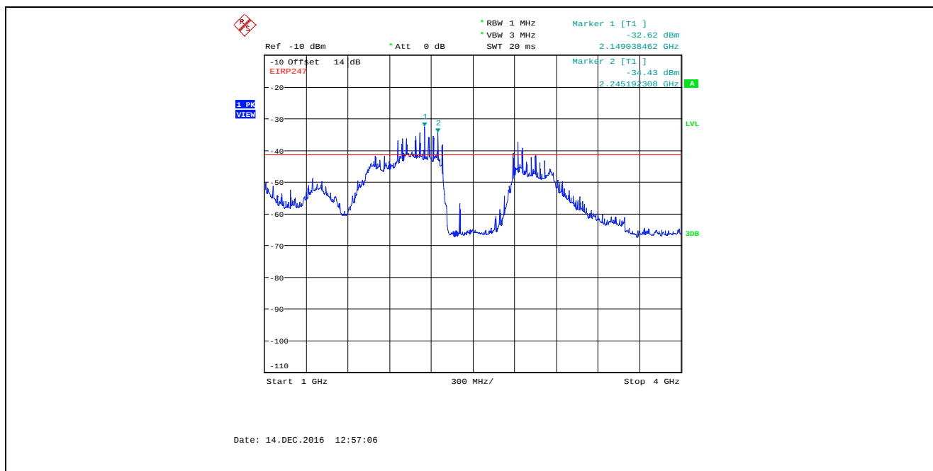
Plot 5.4.4.3.4. Conducted Spurious Emissions in Restricted Frequency Bands Channel 1, 2405 MHz, MSK Modulation, Power Setting 12, 1 GHz - 4 GHz, Peak Detector
