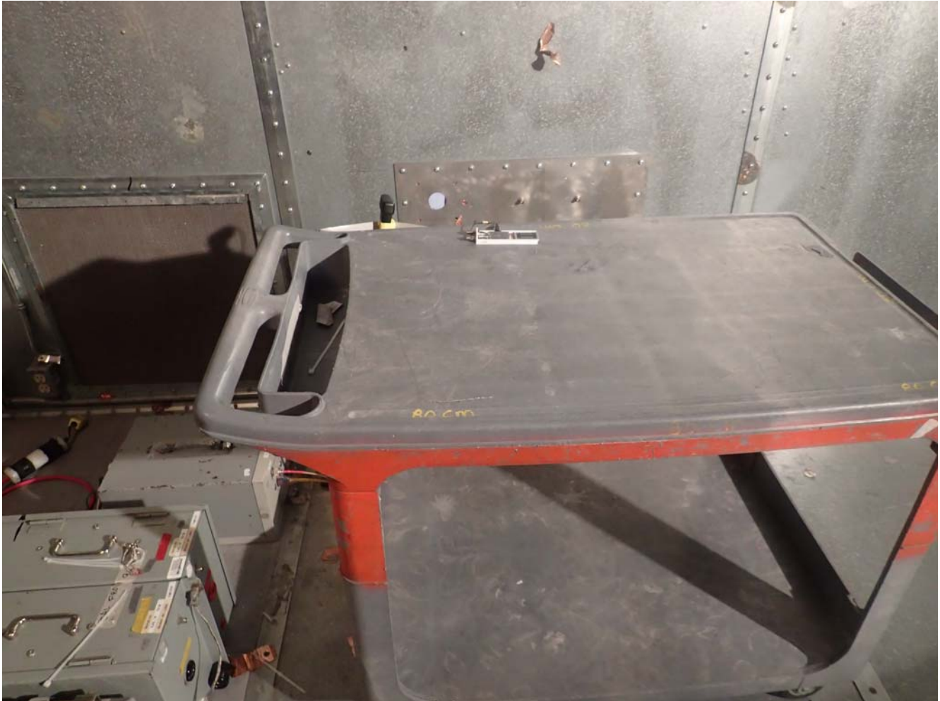
Power Line Conducted Emissions Test Configuration 1: 5 VDC Via AC Adapter
