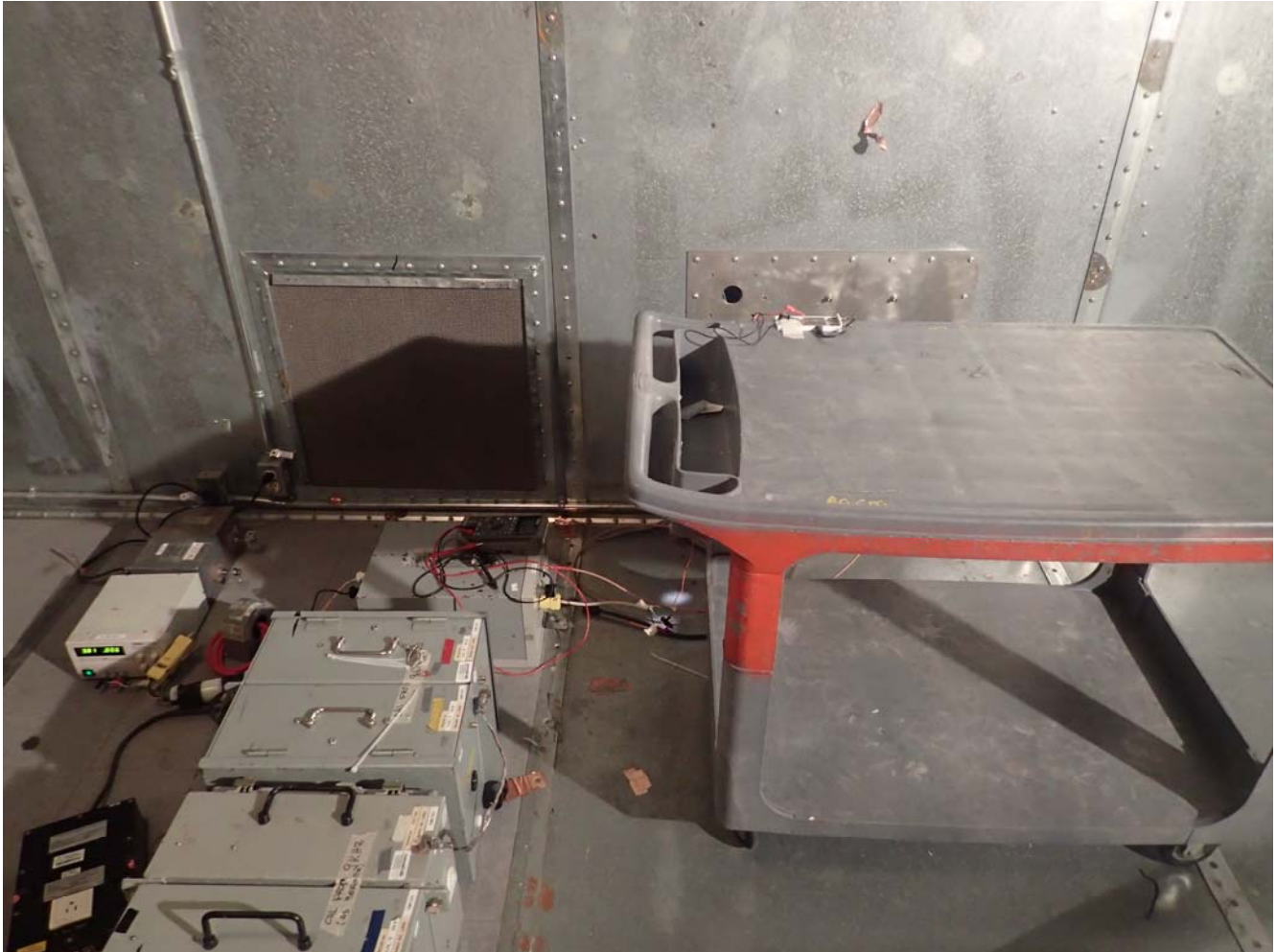
Power Line Conducted Emissions Test Configuration 2: 3.7 VDC from DC Power Supply
