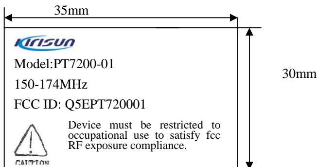
The Label must not be a stick-on paper label. The Label on these products must be permanently affixed to the product and readily visible at the time of purchase and must last the expected lifetime of the equipment not be readily detachable.
