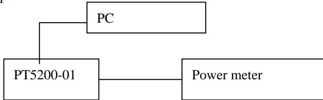
b. running Software:KSP5200V3.04, set the power to 3.5W
