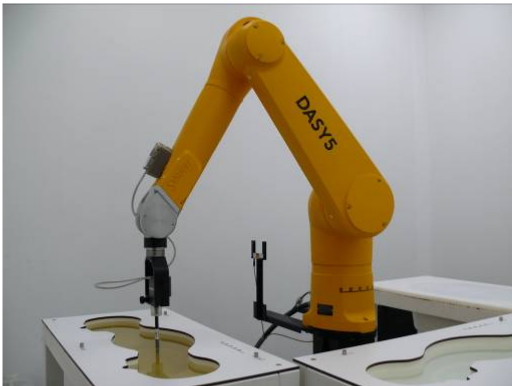
Picture 1: Specific Absorption Rate Test Layout
