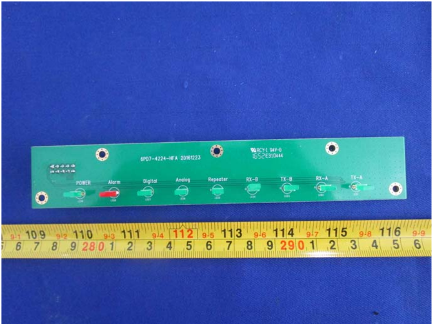
EUT – Led Board Top View
