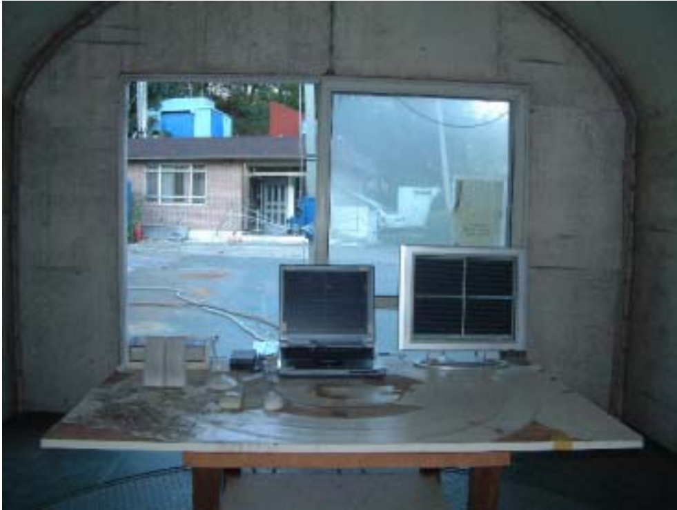
RADIATED EMISSION SETUP PHOTOGRAPH - FRONT VIEW ( 30 - 300 MHz )
